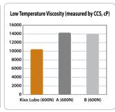
The lower the viscosity, the higher the fluidity of engine oil is mainteind at low temperature. Therefore, the smooth operation of automotive engines is possible in cold area.
